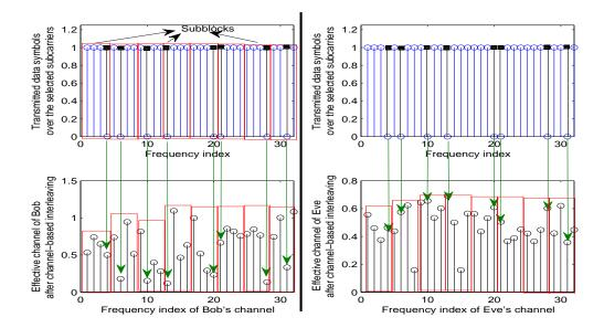
Fig. 3. Subcarrier structure of the designed secure OFDM-SIS-AIS scheme with  $\zeta = 3/4$ : In each sub-block, surrounded by red rectangle, the sub-carriers (blue-colored) experiencing good sub-channel gains with respect to Bob are used for data transmission, while the rest (black-colored) are injected with AIS. Note that with respect to Eve, the AIS-injected sub-carriers do not usually correspond to her weak (bad) sub-channels as apposed to Bob's subchannels.
