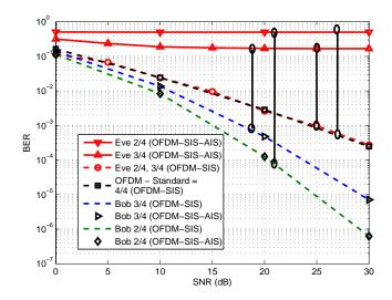
Fig. 4. BER performance comparison between Bob and Eve when OFDM-SIS-AIS is used compared to OFDM-SIS. QPSK modulation alongside  $\zeta=3/4$  and  $\zeta=2/4$  are adopted. TDD mode is considered, where Eve does not know Bob's CSI [6].
