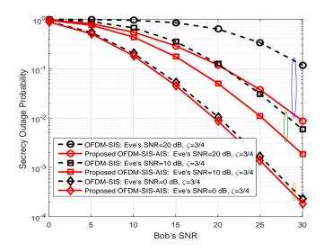
Fig. 6. Secrecy outage probability of the proposed OFDM-SIS-AIS for  $\bar{\gamma}_e=0,10,20$  dB,  $\zeta=3/4$  and  $R_s=1$  compared to conventional OFDM-SIS.
