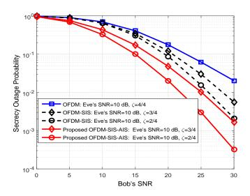
Fig. 5. Secrecy outage probability of the proposed OFDM-SIS-AIS for  $\zeta = 1, 3/4, 2/4, \bar{\gamma}_e = 10$  dB, and  $R_s = 1$  compared to conventional OFDM-SIS.
