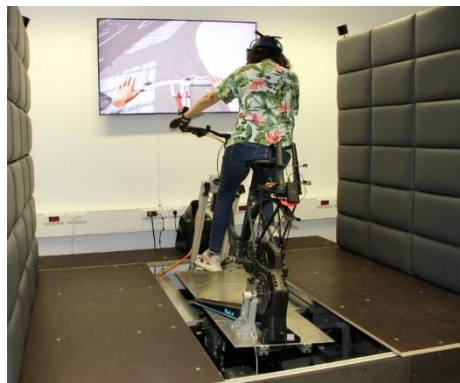
Figure 1. Bicycle simulator at the MoSAIC-VRU-Lab from the German Aerospace Center (DLR)
