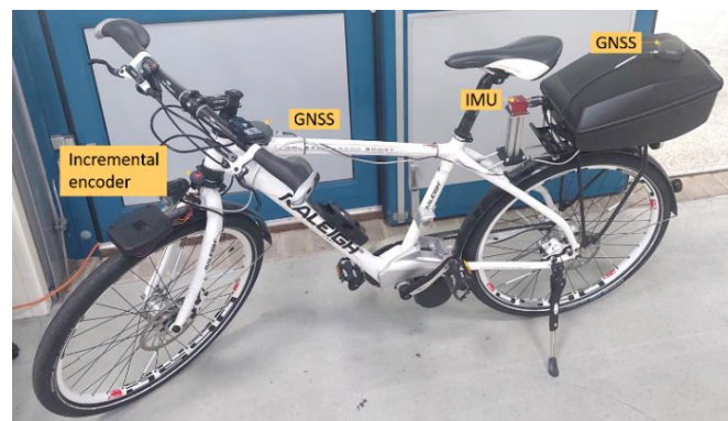
Figure 4. Research bicycle instrumented with sensors
