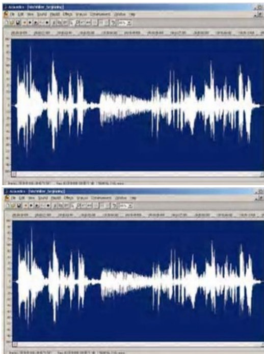
Fig. The signal level comparisons between a WAV carrier file before (above) and after (below) the LSB coding is done [9]
